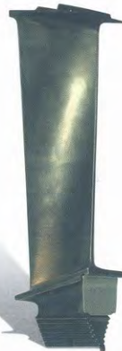
Second stage blade 12MW/500 gr
