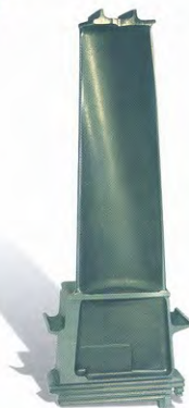
Second stage blade 38MW/2.5 Kg
